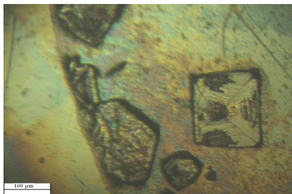
Figure 1 – Surface outgrowths after local treatment by solution
